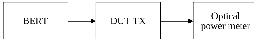
Figure 2- 7 Average optical power test
