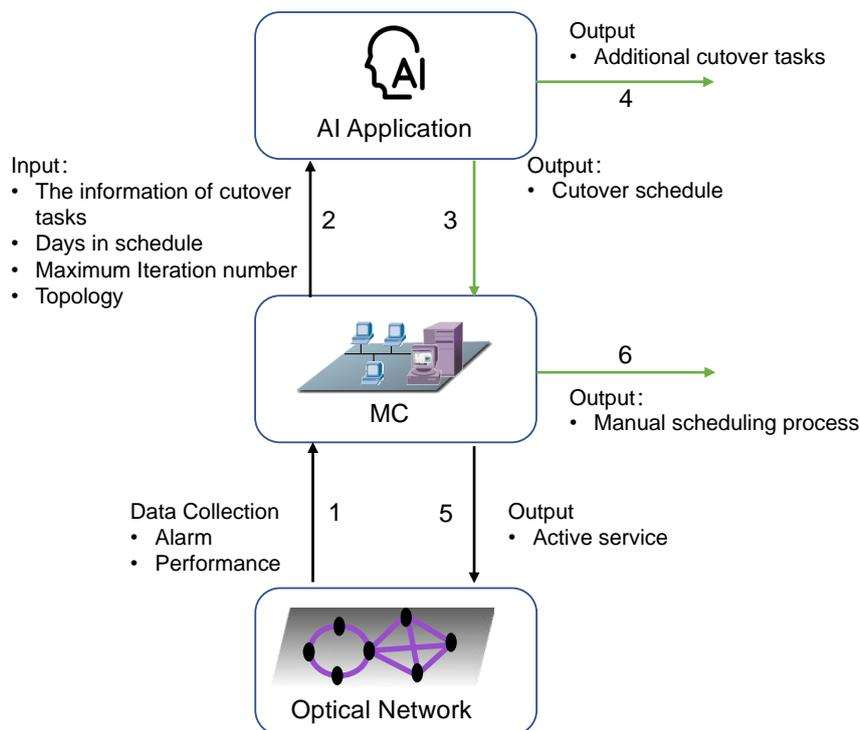
Figure 10 Architecture of intelligent task scheduling for optical cutover
