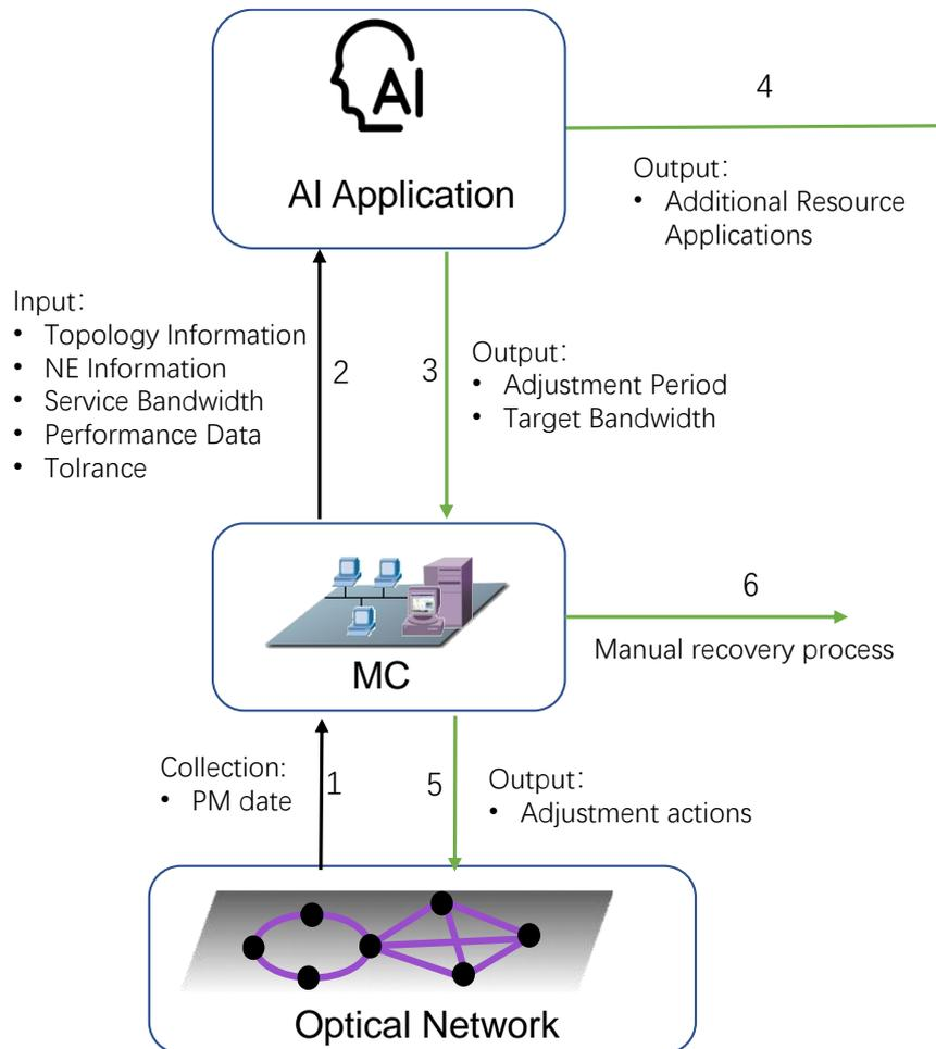
**Figure 5 Architecture of Intelligent Traffic Prediction**
