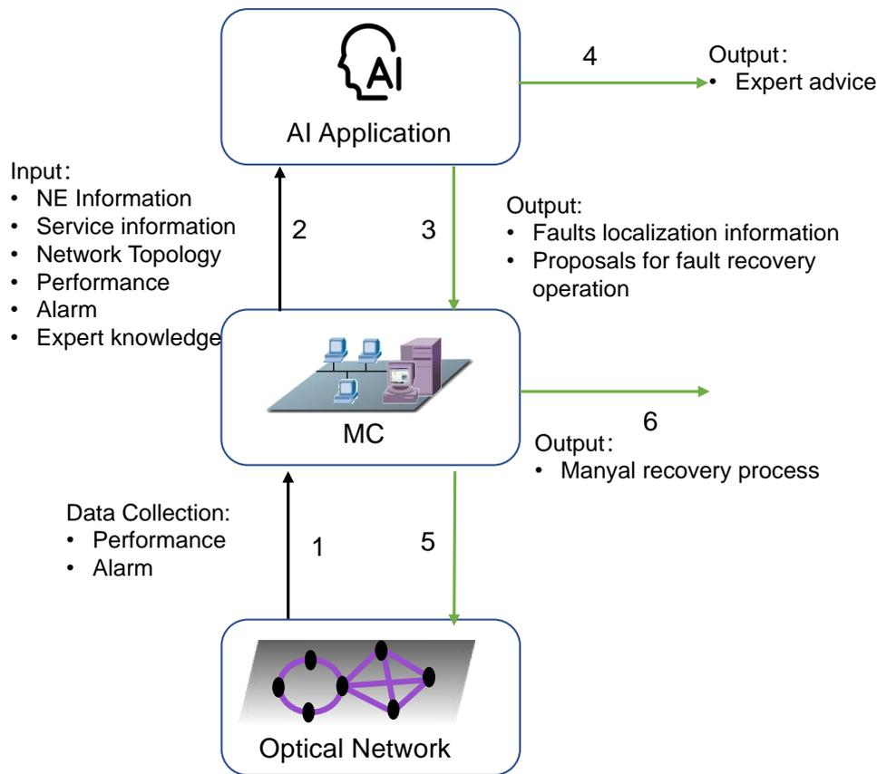
Figure 2 Architecture of Intelligent faults localization
