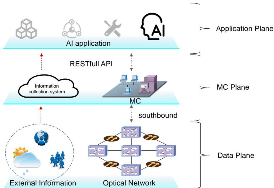
**Figure 1 Architecture of AI application in optical network maintenance**
