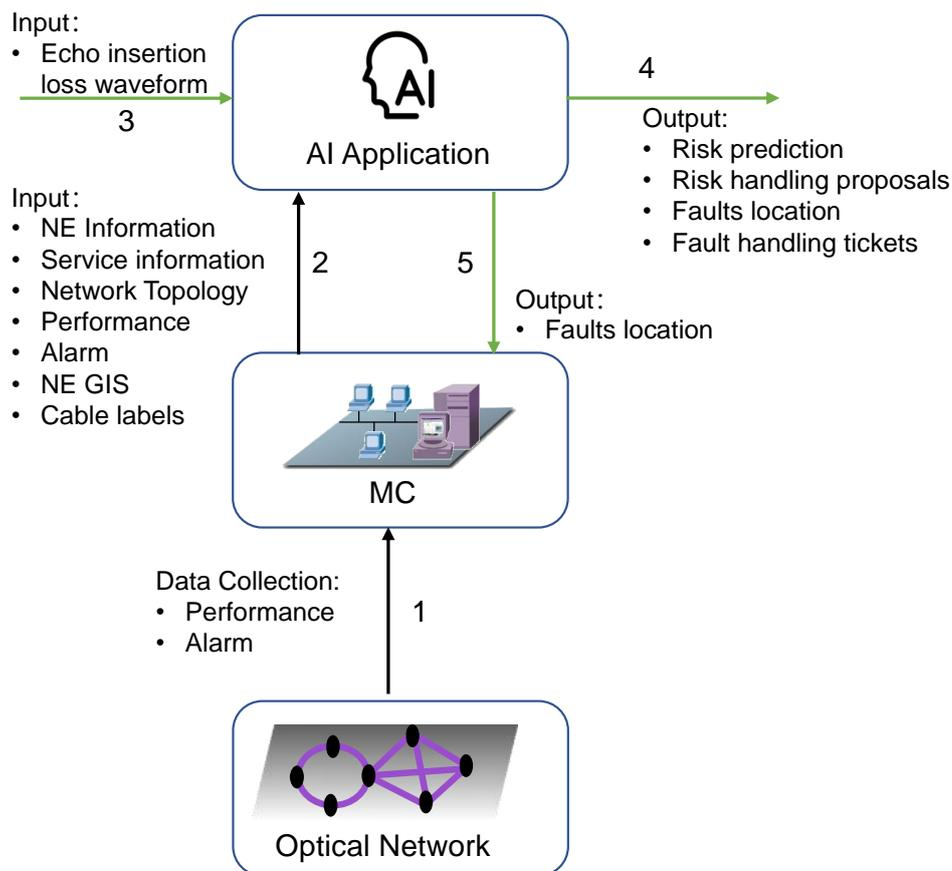
Figure 9 Architecture of intelligent Pre-warning for cable breakage-proof
