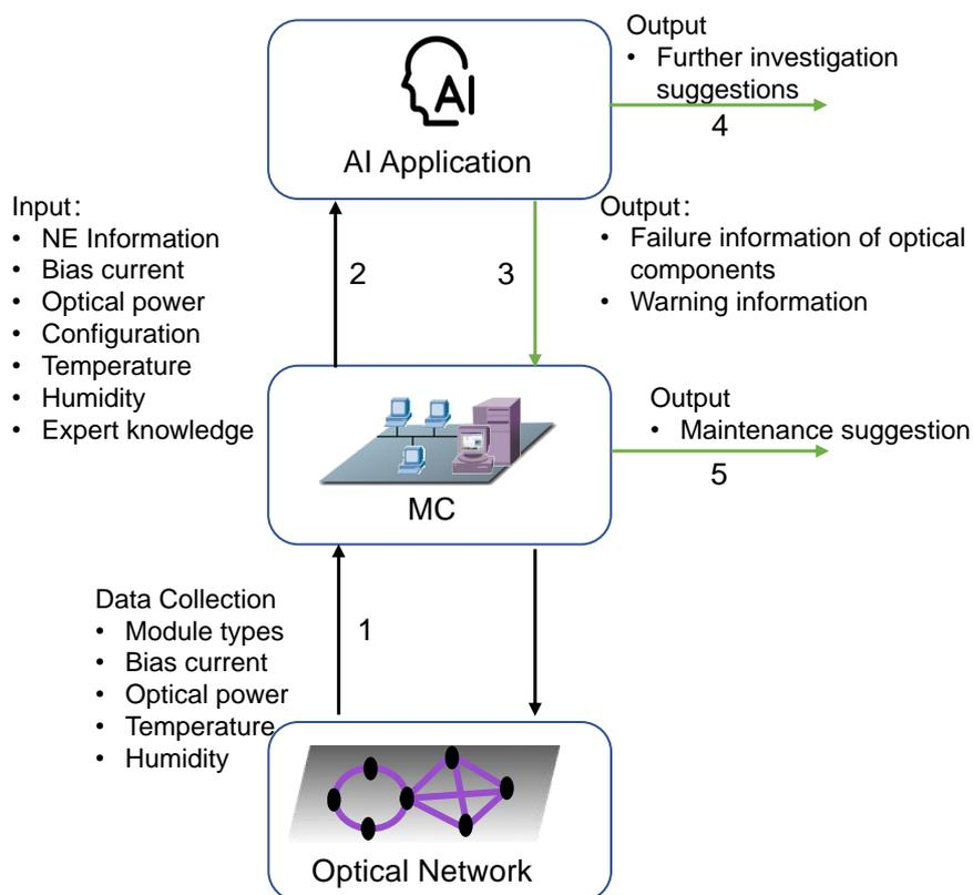
**Figure 3 Architecture of Intelligent prediction of optical component failure**
