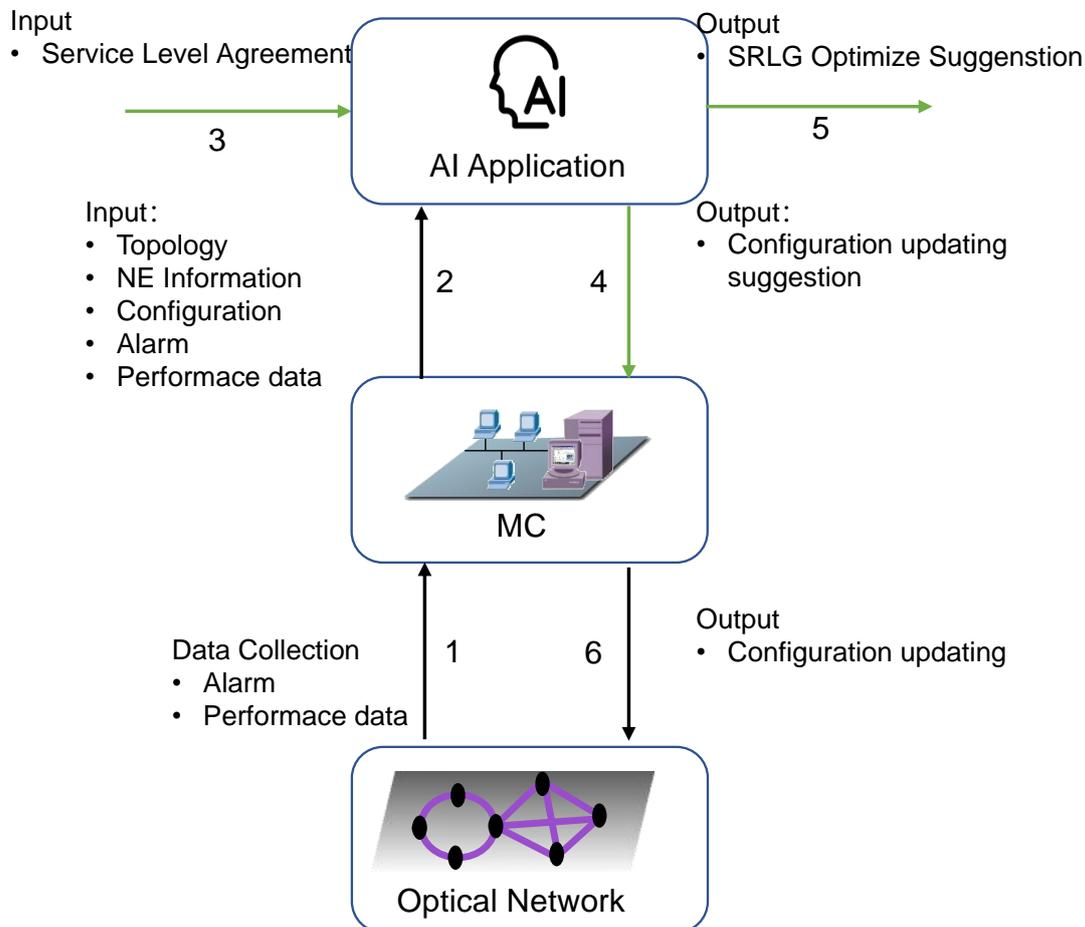
**Figure 6 Architecture of detection and optimization of SRLG**
