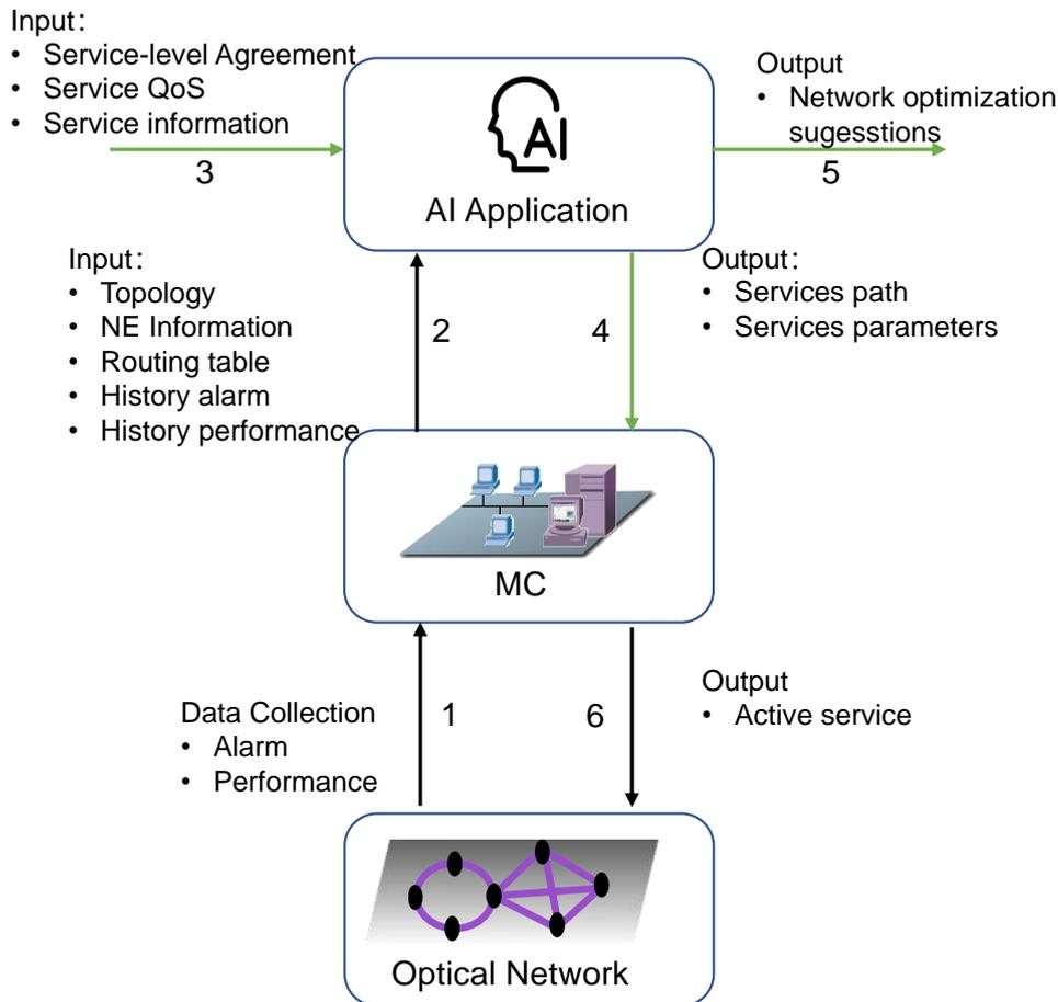
**Figure 7 Architecture of service intelligent configuration**
