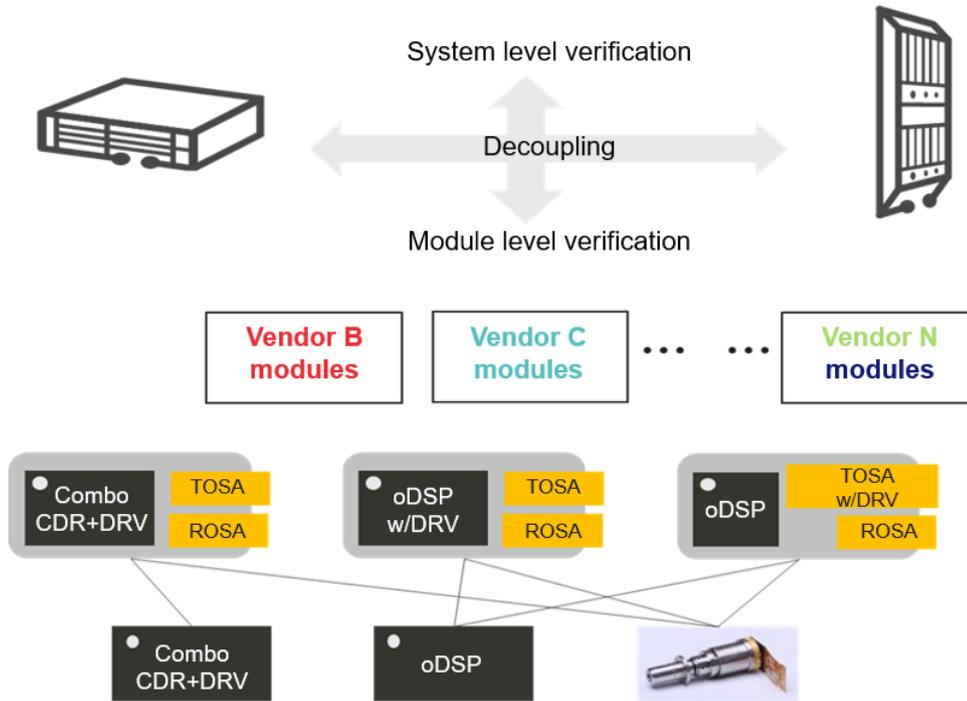
Figure 17 Decoupling of the optical module test from the main device test
