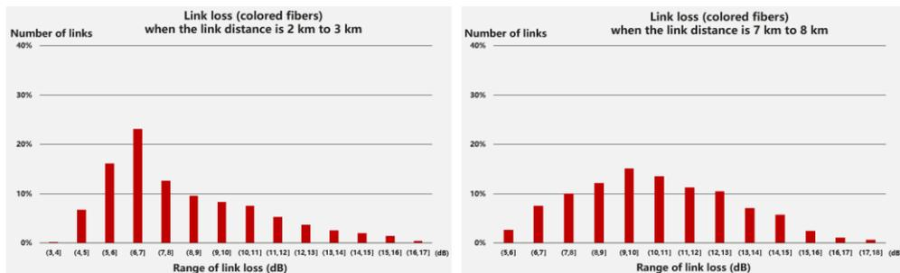
Figure 6 Distribution of link loss with WDM optical modules under different link distance ranges
