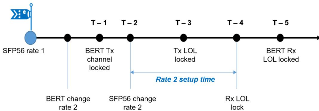
Figure 15 Rate switching setup time test
