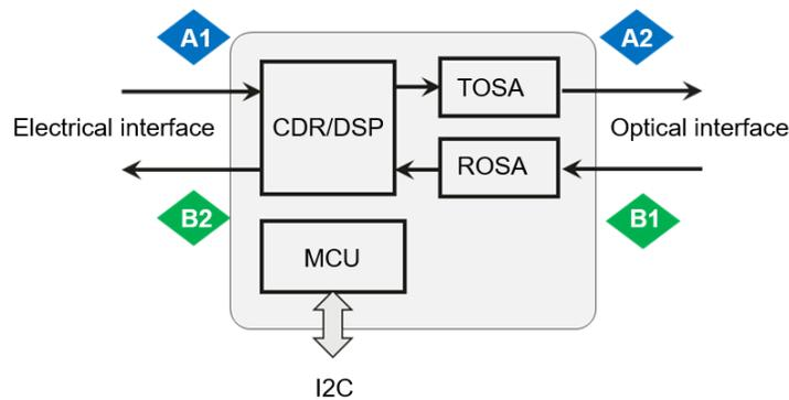
Figure 14 Logical diagram of the rate switching setup time test
