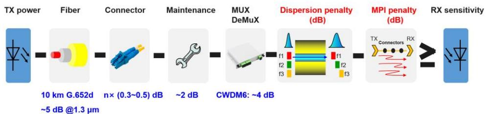
Figure 4 Link budget for CWDM optical modules
