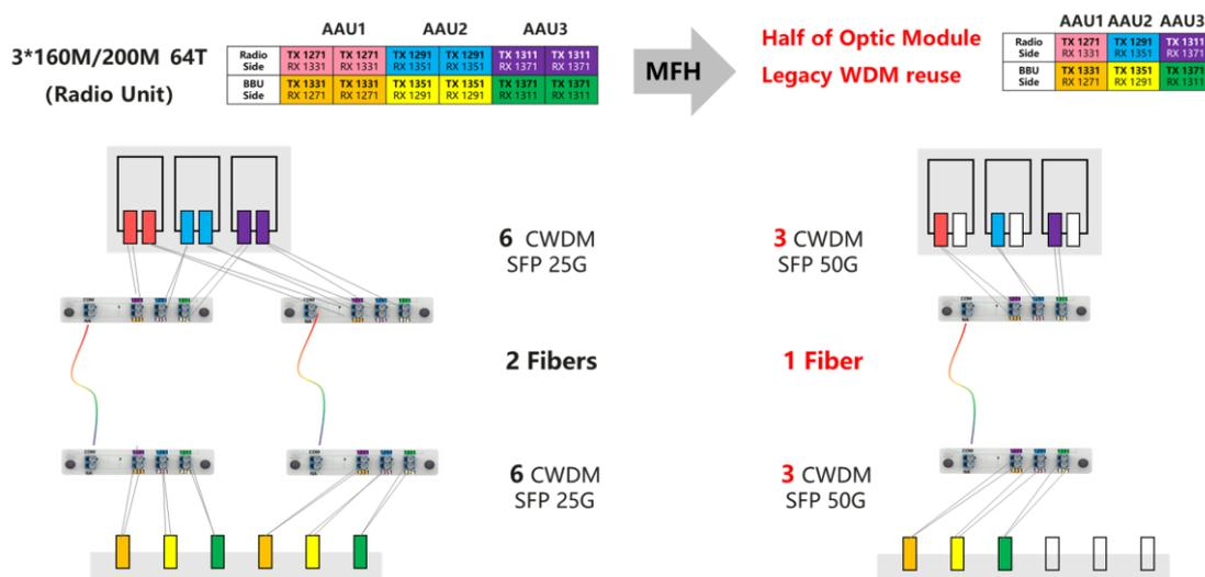
Figure 11 Wireless fronthaul evolution solution
