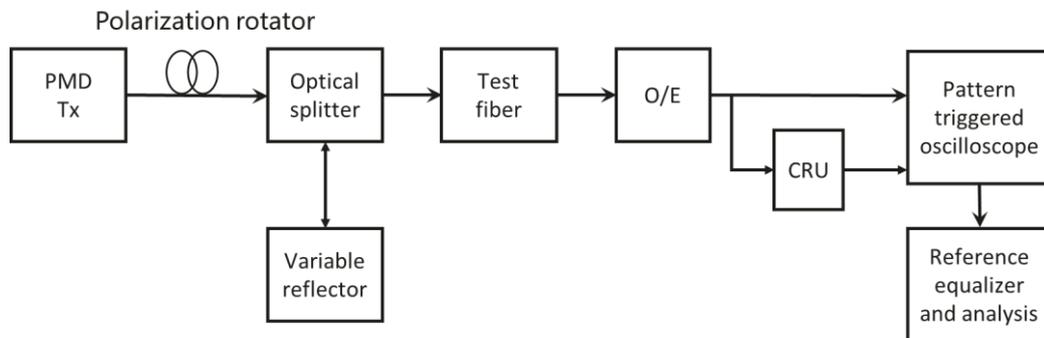
Figure 12 TDECQ test networking (source: IEEE Std 802.3cd™-2018)
