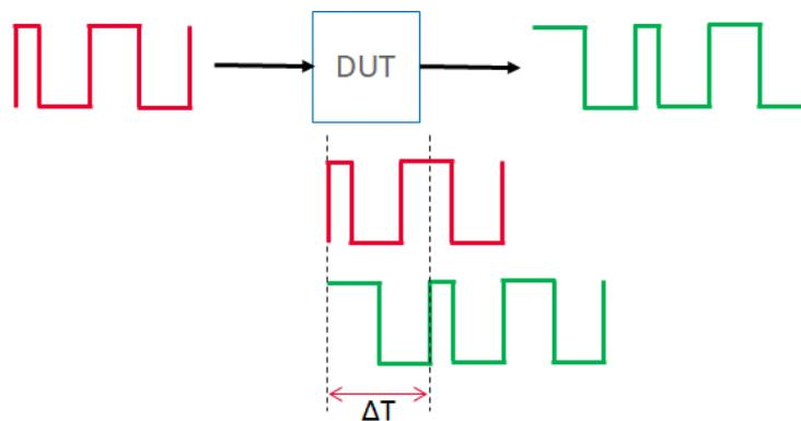
Figure 16 Latency test
