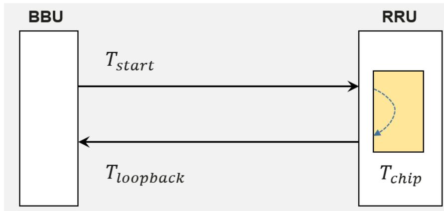
Figure 2 Measurement of the transmission distance of an optical fiber
