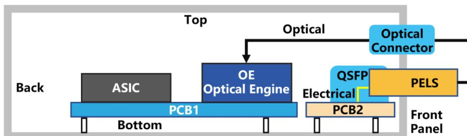
Figure 1.3 Concept of PELS with QSFP like and Optical Connector on the both sides
