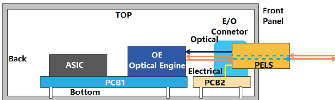
Figure 1.5 Concept of OE TRx optical interface integrated on the PELS module
