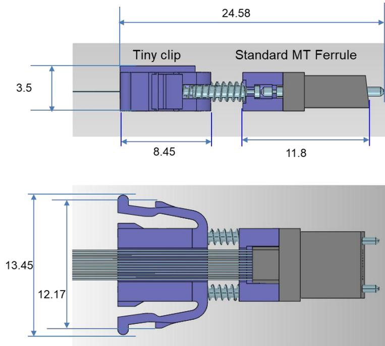
Figure 5.3 Details of host optical connector with clip and spring
