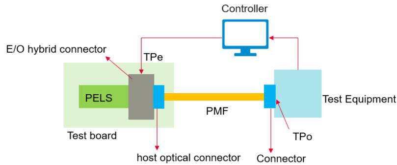
Figure 9.1 OIO PELS test points
