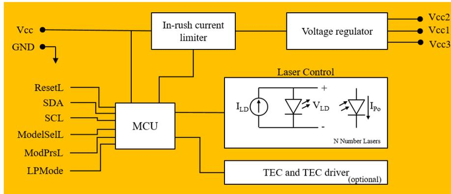
Figure 4.2 Electrical block diagram of a PELS module
