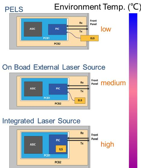
Figure 1.2 Three solutions of source and its environment temperature.
