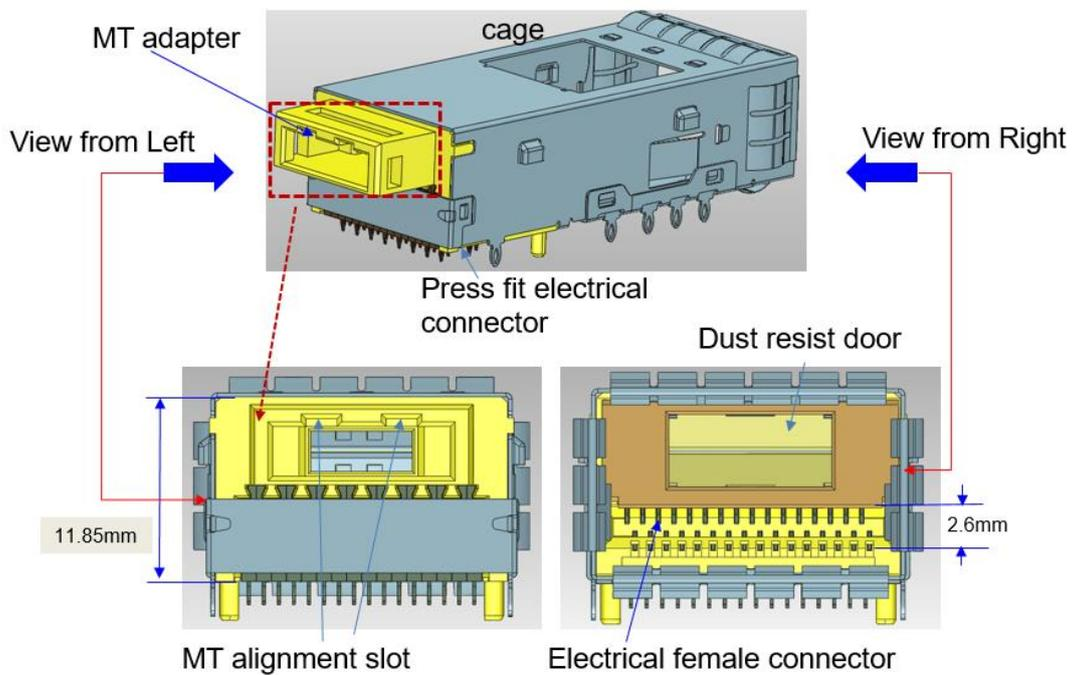
Figure 5.2 Detailed of E/O hybrid connector and cage
