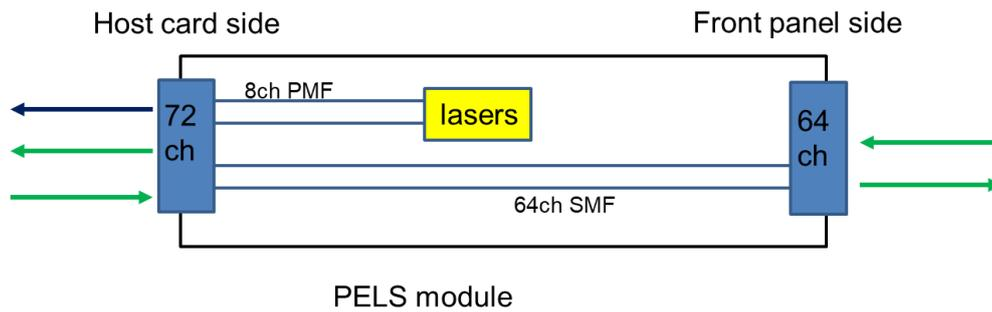
Figure 1.6 Concept of pass-through PELS module
