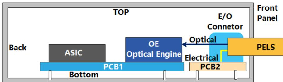
Figure 1.4 Concept of PELS with Electrical/Optical Connector on the same side
