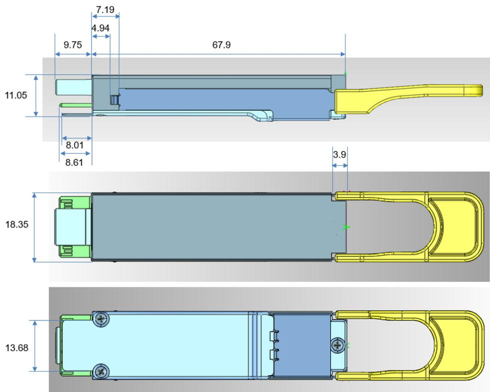
Figure 2.3 Detailed size parameters of type-A OIO PELS
