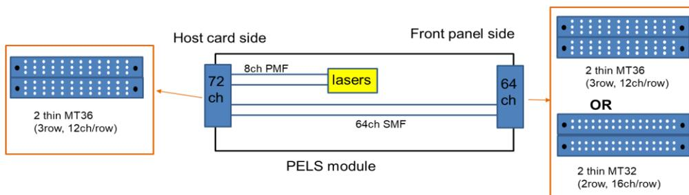
Figure 3.3 PEELS with Pass-through design
