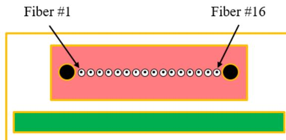
Figure 3.2 PEELS MT-16 Ferrule output endface for 16ch optical channel
