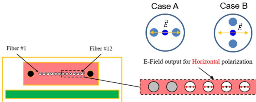
Figure 3.4 Horizontal polarization of OIO PEELS. Case A: PMF slow axis horizontally aligned; Case B: PMF slow axis vertically aligned;
