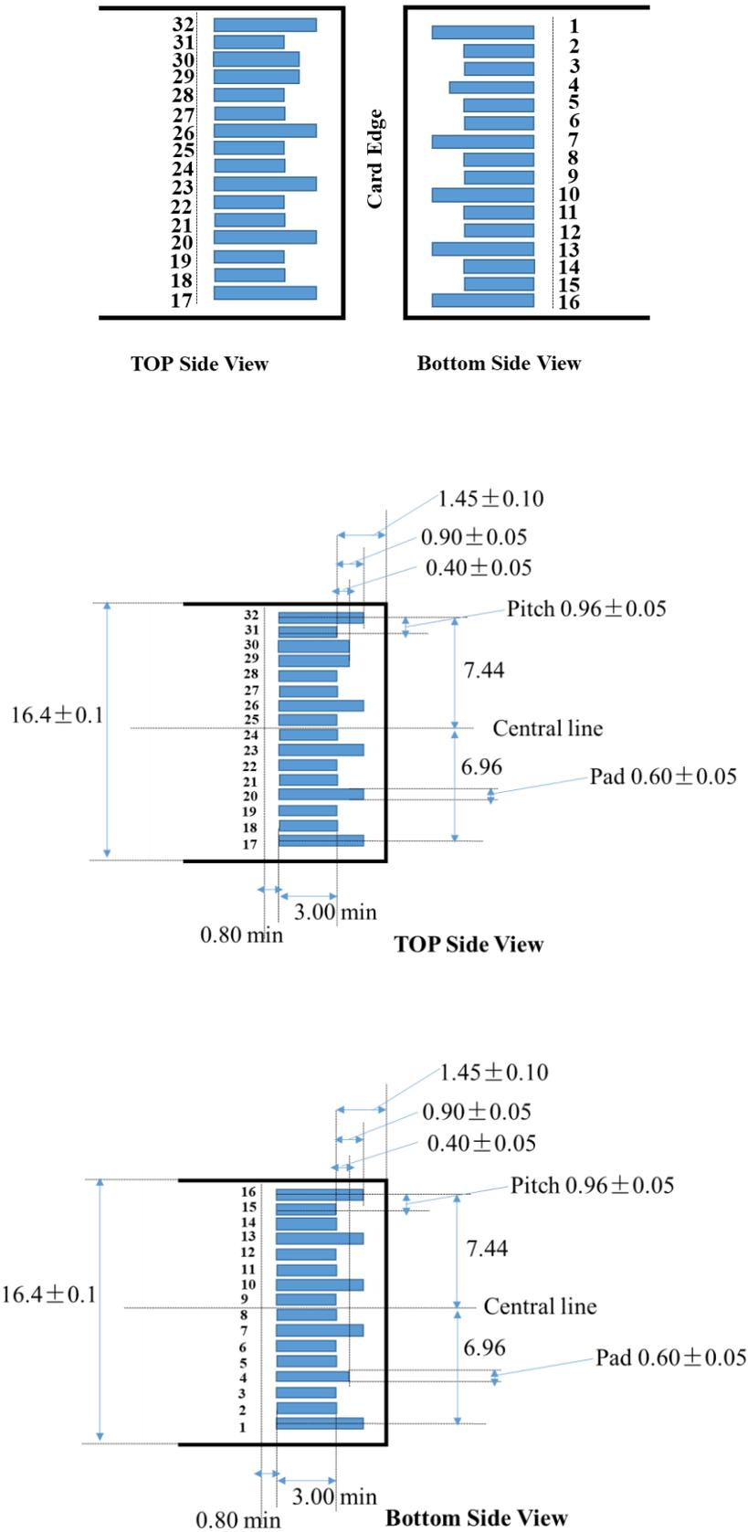
Figure 4.1 Electrical Pin layout view from top and bottom side.
