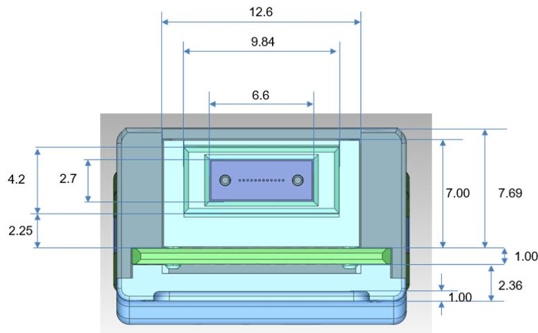
Figure 2.4 Detailed size parameters of optical and electrical interfaces of OIO PELS
