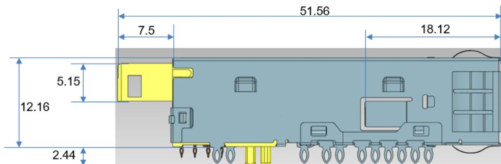
Figure 5.4 Details of host optical connector and cage
