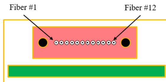
Figure 3.1 PELS MT-12 Ferrule output endface for 12ch optical channel
