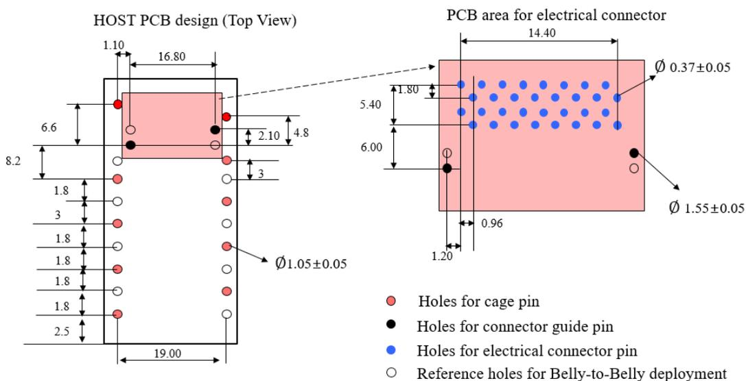
Figure 5.5 Host PCB design layout for PELS belly-to-belly deployment
