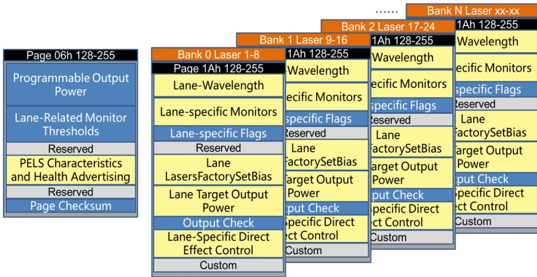
Figure 8.4 page 06h and page 1Ah register section definition
